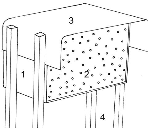
**Fig. 1.** General view of the overwintering chamber. (1) wooden box, (2) fiber-board front side, (3) plastic plate roof and (4) wooden pool
